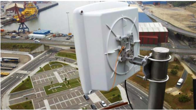
**Figure 6. Device deployed inside an antenna case on Bilbao's harbor controlling railway signaling over a dedicated WPAN.**
